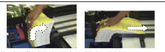
Manually over fill the feeder, then draw the material back over the in-feed conveyor. This will establish a natural radius for the material to follow and provide a starting reference point to position the height sensor. (*Fig. 17*)
